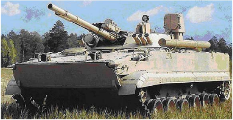
Figure 3-7-29: The BMP3 ICV has Three 7.62 mm PKT Machine Guns, One Mounted Coaxially with the 100 mm gun and 30 mm Cannon in the Turret and one on Either Side of the Bow Firing Forwards (Jane's 2000)
